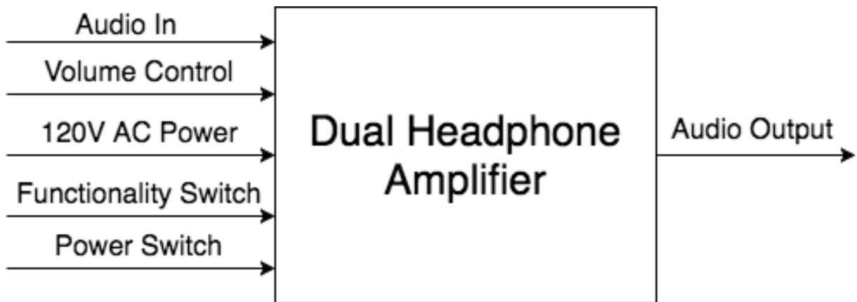
Figure 1: Level 0 Block Diagram of the Dual Method Headphone Amplifier
