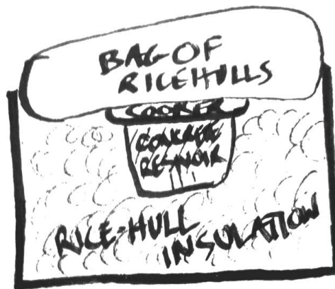
Figure 11. This concept consists of a cylindrical concrete reservoir with a rebar heater immersed in the center and welded to the cast iron cooking surface. Rice hulls would surround the reservoir and a bag of rice hulls would insulate the top.
