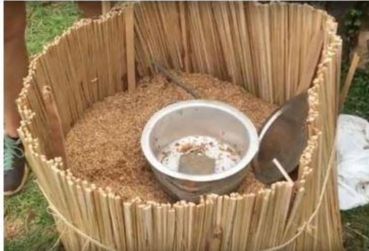
Figure 6. ISEC implemented in Uganda. The outer structure is made of reed mat and rice hulls are used as insulation. The heater rests inside a larger pot and a smaller pot holding food rests on top the heater. A ceramic tile is placed under the larger pot to insulate rice hulls from hot spot under the heater. (Watkins et al. 2017).
