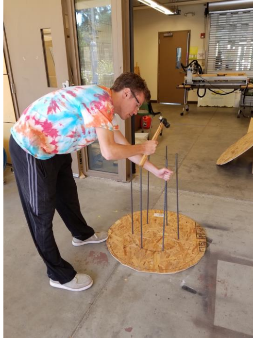
Figure 26. Kyle hammers the rebar poles into the housing base.
