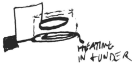
Figure 13. This idea focuses on the heating element and includes a thermal switch to direct the power to a heater either immersed directly in the food or one in the thermal storage.
