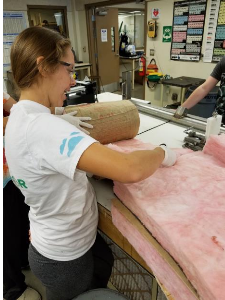
Figure 34. Amanda cheerily cuts fiberglass insulation to be used on the housing unit lid and beneath the thermal reservoir.
