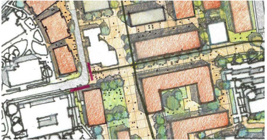
Figure O: Pedestrian Hybrid Beacons shown in maroon on Perimeter Road and University Drive alongside proposed bike lane in dark green, overlaid on a Master Plan Conceptual Map
