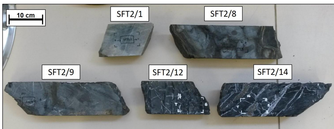
Figure 5.83: Samples sent for thin section cutting – SFT2/1, SFT2/8, SFT2/9, SFT2/12 and SFT2/14. Note that SFT2/8 could not be cut into thin section due to its weathered nature.
