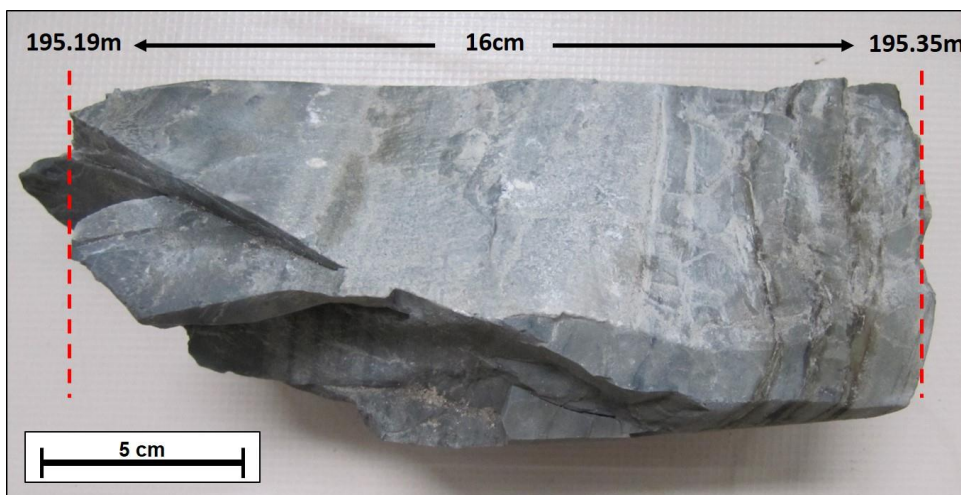
Figure 5.61: Cherty layer at 195.19m – a possible correlation to the 'Matjiesfontein chert' as described by Visser (1992).
