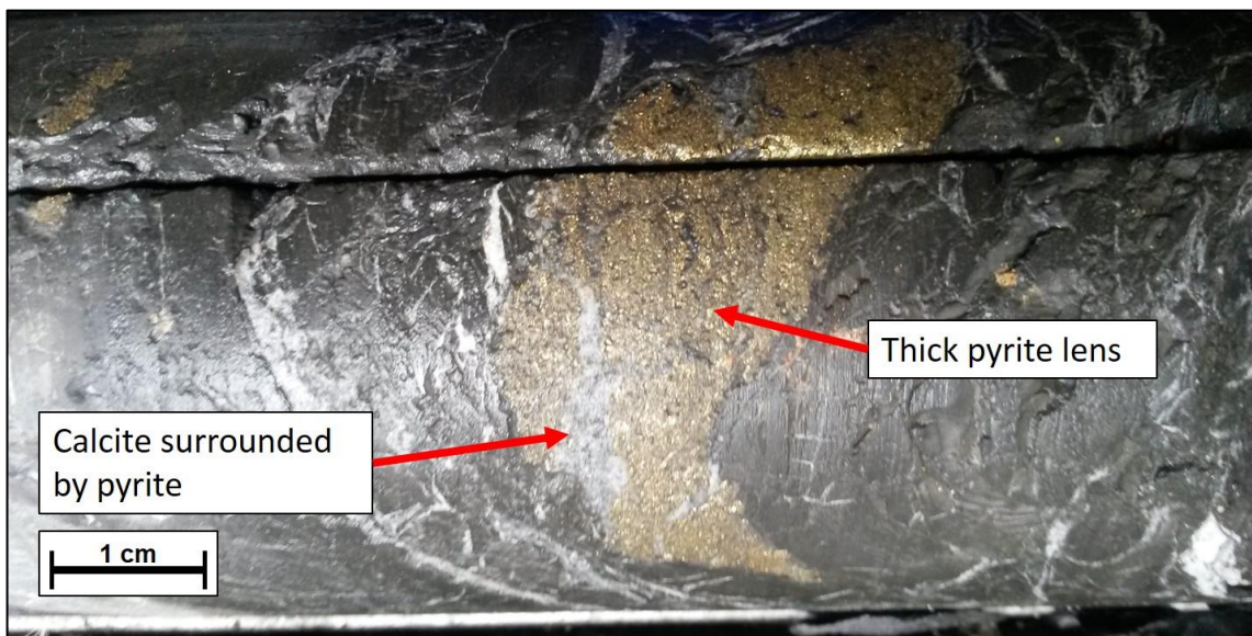
Figure 5.72: Thick pyrite lenses associated with randomly orientated calcite veins. Contacts between the areas rich in calcite and pyrite seem to be represented by thrust faults which separate them from the homogeneous black shale.
