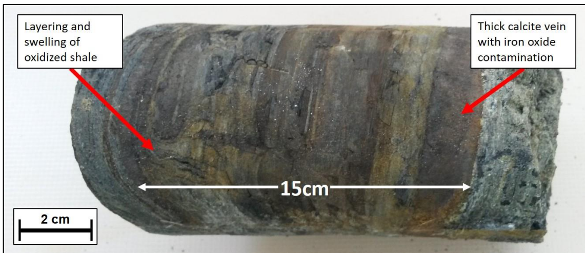
Figure 5.78: Discolouration and swelling of shale caused by oxidation of pyrite. The outer layers are calcite veins which have been contaminated by iron oxide.
