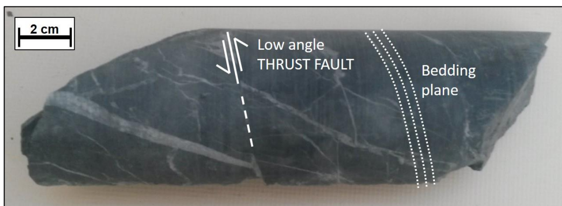
Figure 5.81: Black shale intersected by randomly orientated calcite veins which are offset by low-angle thrust faults.
