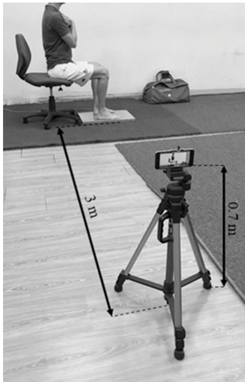
Fig. 1. Measurement environment. iPhone positioned on a 0.7 m-high tripod placed 3 m from the right side of the participant.
