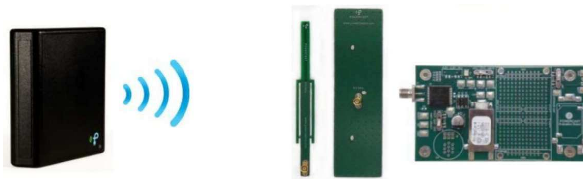
Figure 18: P2110-EVAL-01 RF Energy Harvesting Development Kit [Ref. 13].
