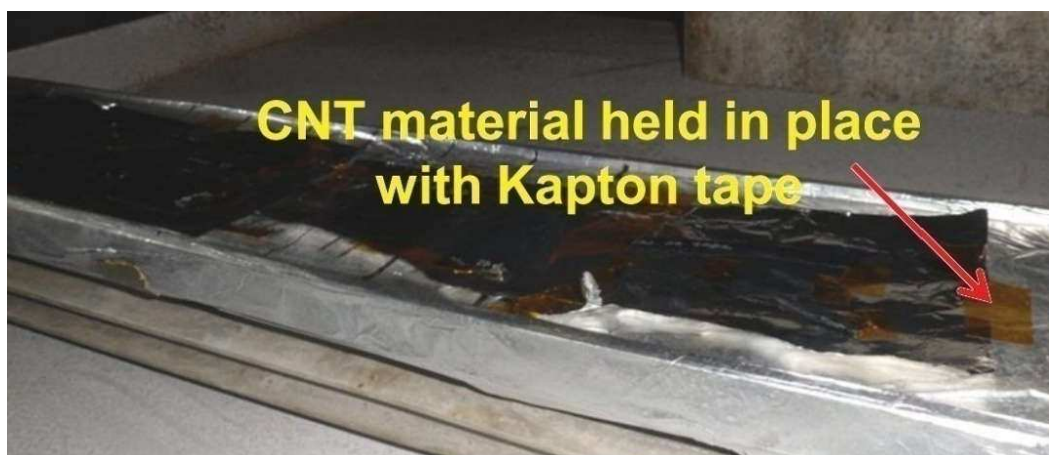
Figure 44: CNT application on the space material [Bib. 9].
