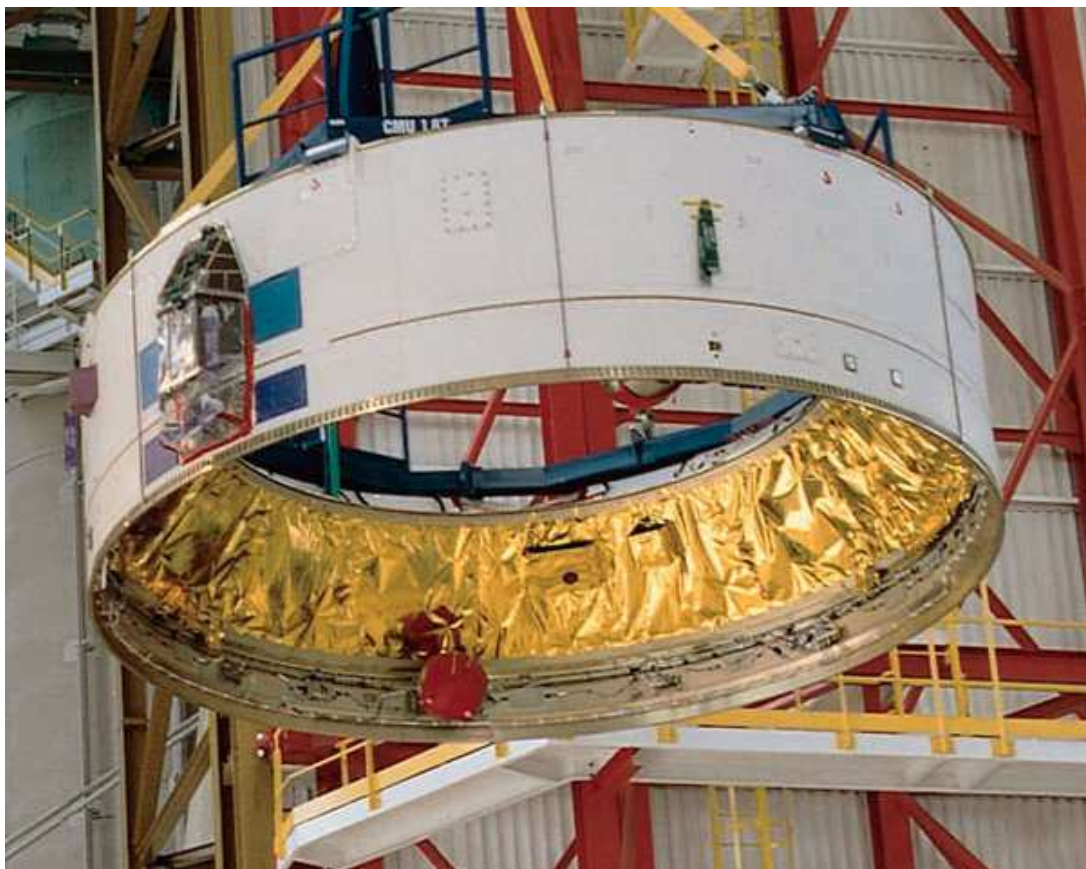
Figure 50: MLI material on the VEB [Ref. 4].
