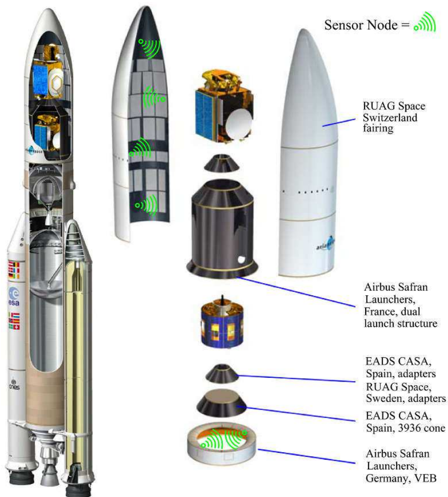
Figure 2: The wireless sensor node placement for Ariane 5 upper stage [Ref. 3].
