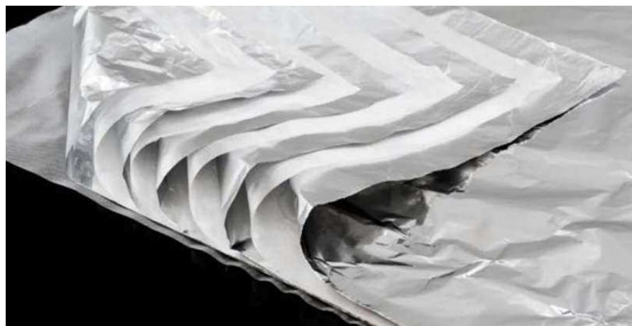
Figure 46: MLI physical view for cryogenic hydrogen tanks [Ref. 50].
