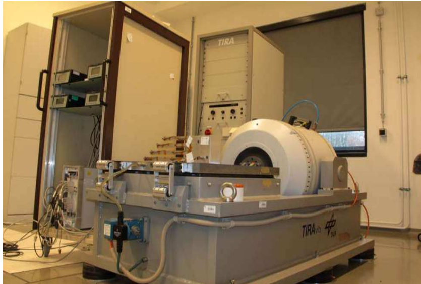
Figure 102: Test equipment for sinusoidal test in German Aerospace Centre Bremen [Ref. 68].
