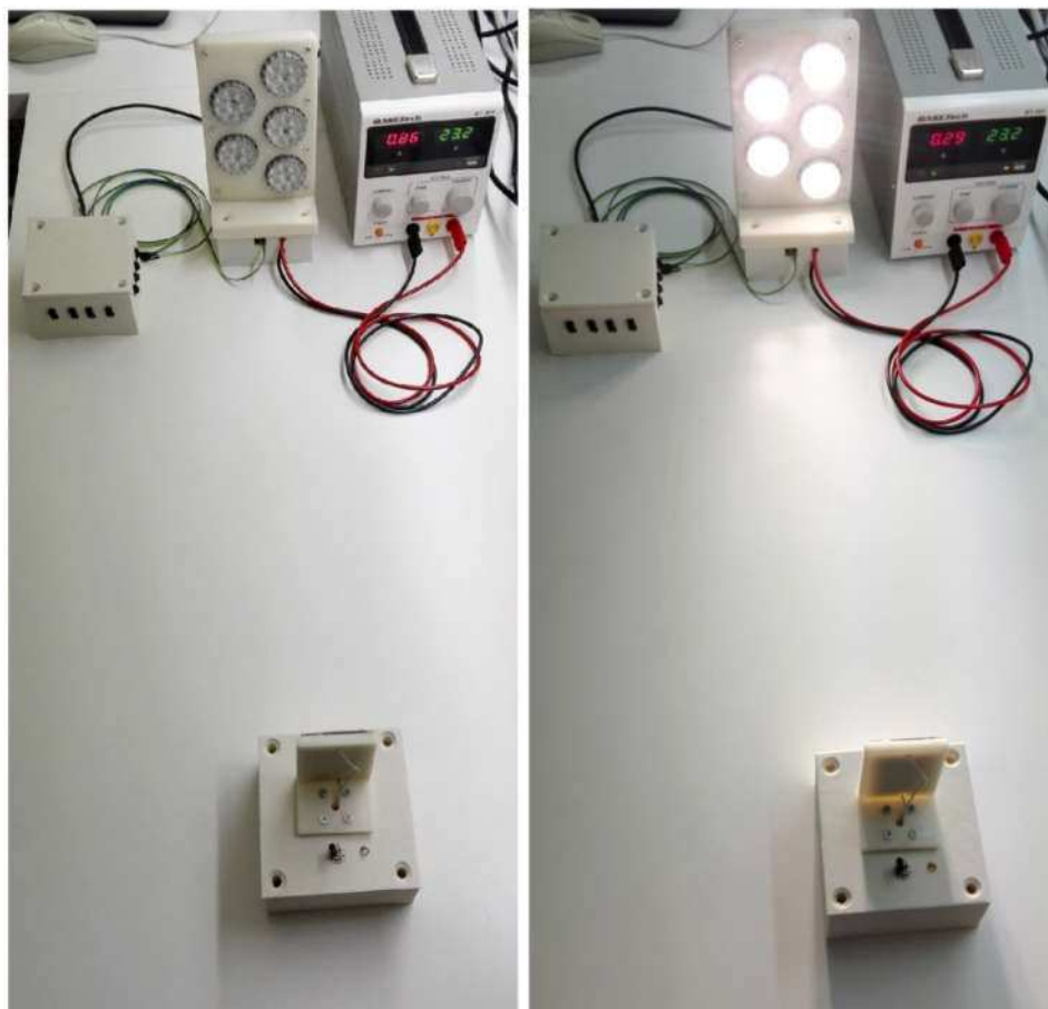
Figure 101: Infrared receiver and VLC transmitter redesigned casings.
