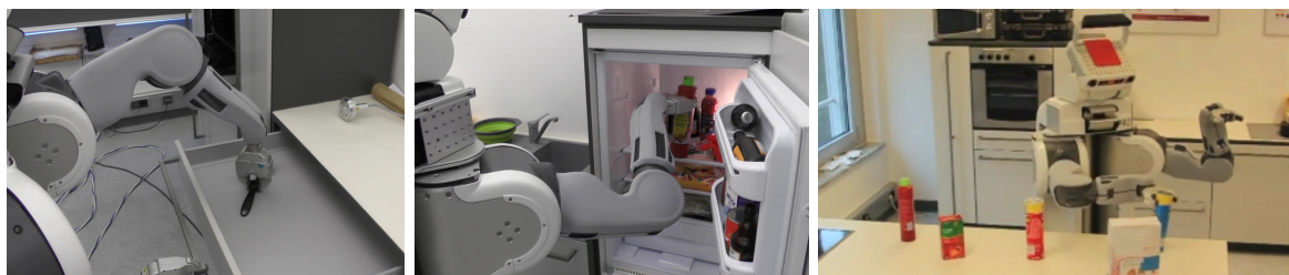
Figure 1.8: Picking objects in different situations: Objects can be stored in drawers or fridges that need to be opened and that act as collision objects; places can be crowded with objects, and every detected object needs to be identified, and accounted for during collision checking.
