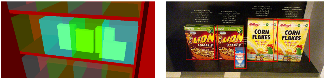
Figure 1.2: Precise environment knowledge is an enabler for reasoning-intensive plans. It does not only store and infer correct object identities and poses, but also discovers multiple instances of the item to pick — triggering decision processes.
