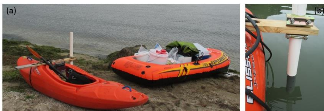
Figure 3.2. (a) Sonde profiler mounted on kayak in white pipe. (b) Instrument in-situ during sampling.
