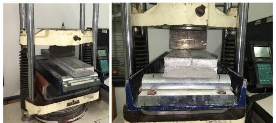
Figure 5-7 FC-N specimen under three-point negative bending test
