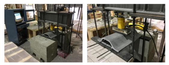
Figure 3-25 Shear specimen SC-S under testing load
