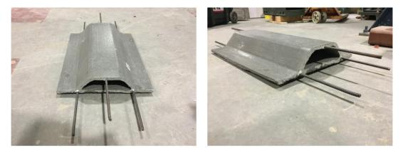
Figure 3-23 Shear specimen (SC-S)
