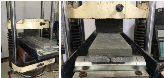
Figure 5-6 FC-P specimen under three-point positive bending test
