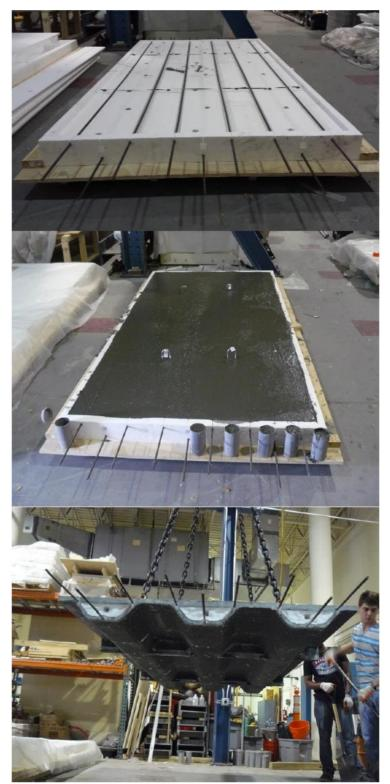
Figure 3-6 Multi-cell specimens preparation
