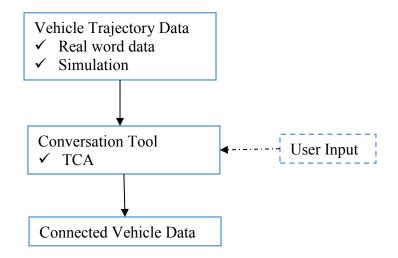
**Figure 4-1: Connected Vehicle Data Emulation Process**
