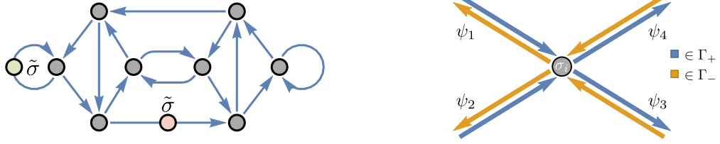
Fig. 3.3.: Right hand side: Illustration of a graph vertex with four attached leads which feature two separate directions, dark/blue and light/orange. Locally the scattering matrix does not couple those directions, e.g. waves entering through an incoming orange edge only leave via an outgoing orange edge, as indicated in Equation (3.3). This ensures unidirectionality on a local scale.
