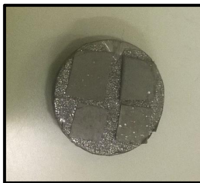
Figure 24 – Sputter-coated fibrous samples with a thin layer of gold.
