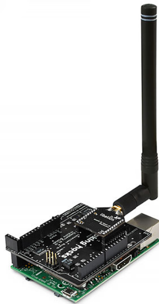
Figure 4.2: Raspberry Pi 2 with Multiprotocol Radio Shield and SX1272 Module
