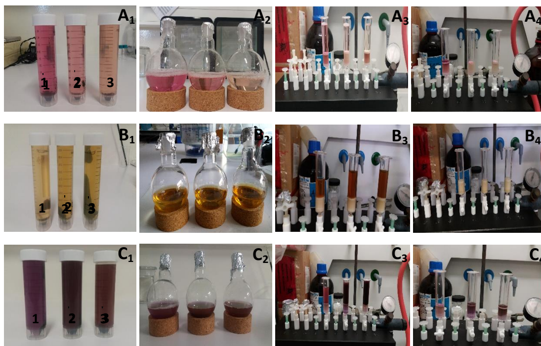
Figure 17: Stages of the cleaning of the extracts of the different species and observation of the different pigmentation during different seasons. A 1-4 : Gracilaria sp. ; B 1-4 : F. vesiculosus ; C 1-4 : P. dioica . 1: Autumn; 2: Winter and 3: Spring
