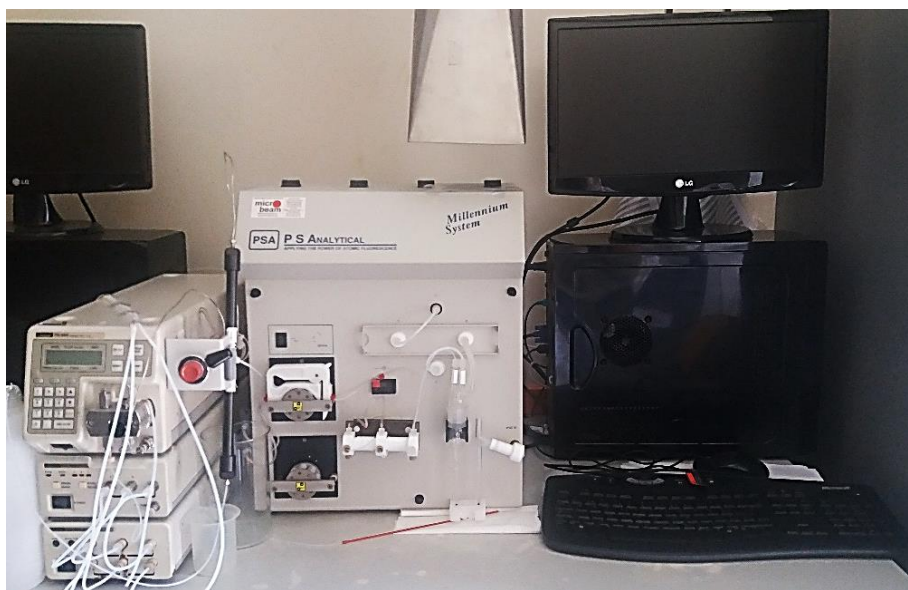
Figure 11: HPLC-HG-AFS system for arsenic speciation
