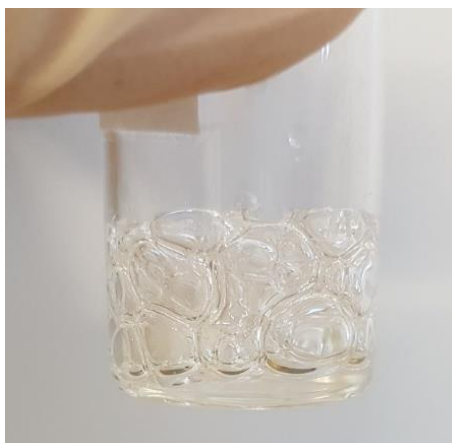
Figure 9: Transparent glassy gel of citric acid, ethanol and \text{Y}(\text{NO}_3)_3 , \text{Yb}(\text{NO}_3)_3 , \text{Er}(\text{NO}_3)_3 , and \text{LiNO}_3 solution.
