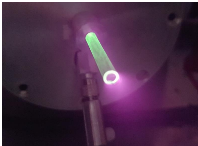
Figure 34: Photograph of Y 2 O 3 : Yb 3+ /Er 3+ nanoparticles doped with 1.1 mol% Li + ions irradiated with a 980 nm laser source with a laser power density of 400 W/cm 2 .
