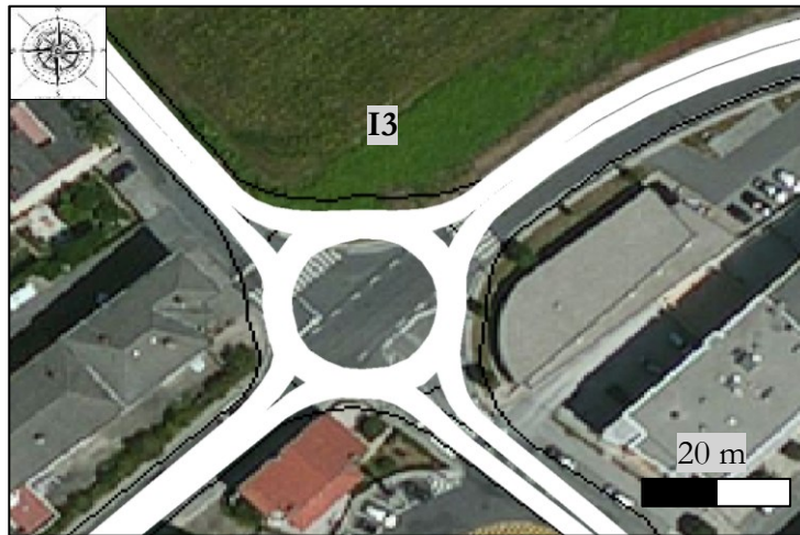
Figure 13 Proposed single-lane roundabout layout at I3 intersection. Source: https://maps.google.com/
