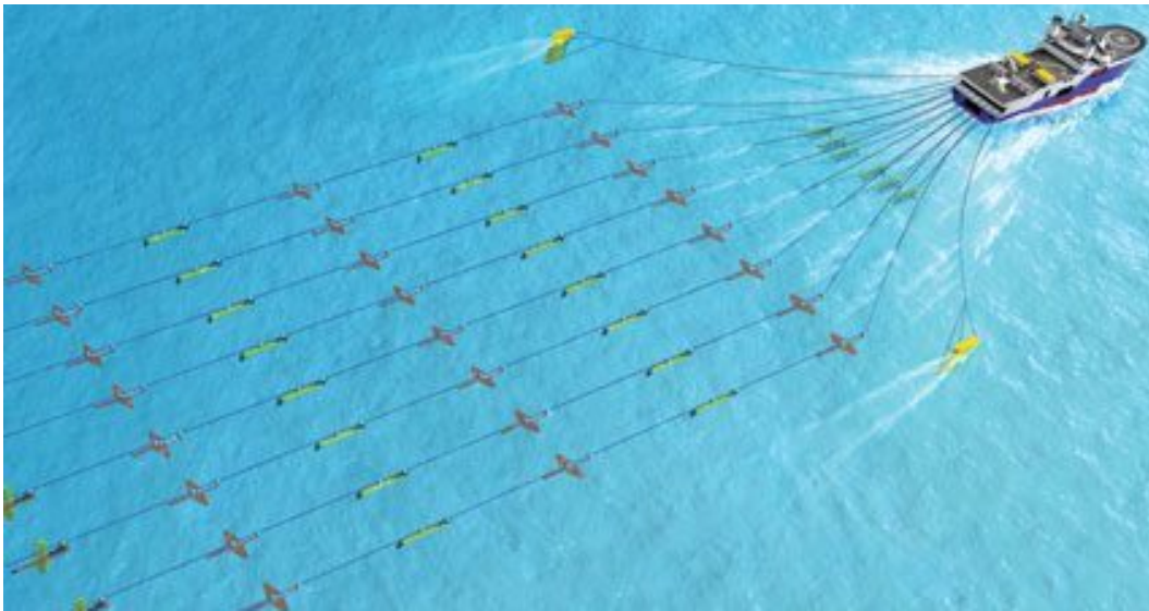
Figure 3.5: Representation of a 3D seismic data acquisition. (Source: http://www.bulwarkservices.com/services/marine-acquisition-system ).
