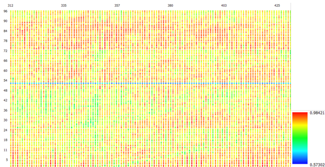
Figure 5.4: "Dead" channel detected in Spectral Comparison - Channel 52, horizontal blue line (horizontal axis represented by FFID and vertical represented by Channel number).
