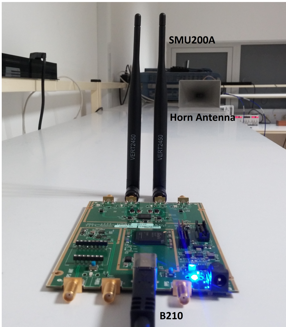
Figure 3.23: Experimental setup for the proposed hybrid detection method evaluation.
