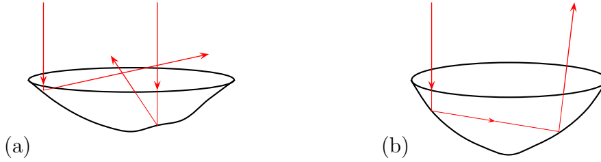
Figure 2: Examples of a function that (a) satisfies and (b) does not satisfy the single impact condition.
