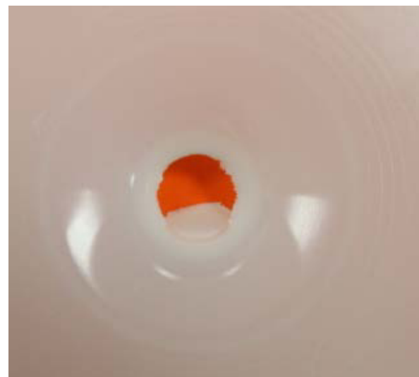
Fig. 5. HDPE deformation after drop weight test at 50 J.
