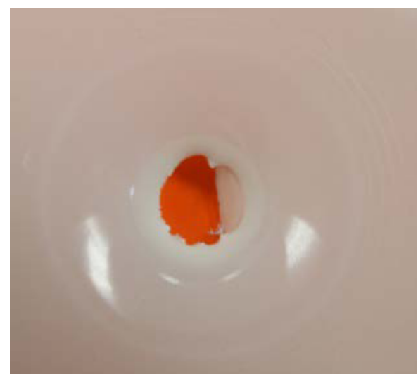
Fig. 6. HDPE deformation after drop weight test at 100 J.
