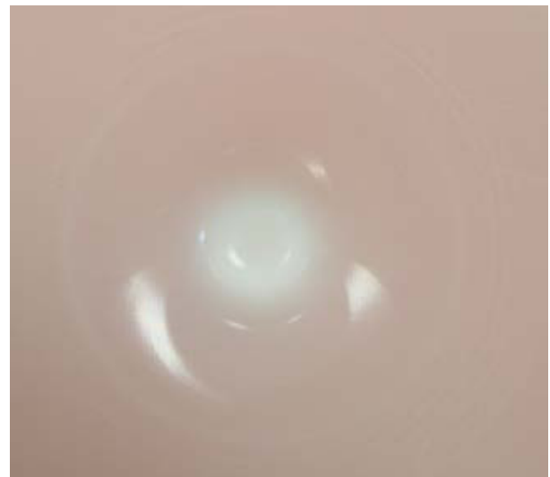
Fig. 4. HDPE deformation after drop weight test at 30 J.
