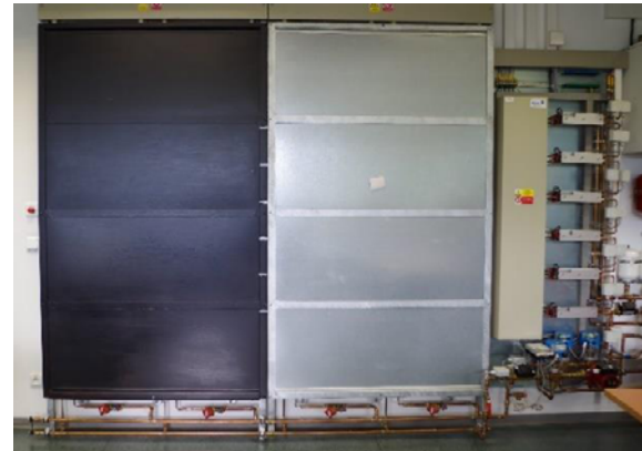
Fig. 4. Thermal panels and thermoelectric assembly on the right.
