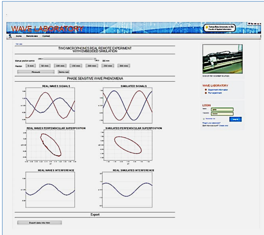
Fig. 4. Example of the view of the RE web page “Remote Wave Laboratory”, measured data, (left) and simulation of the observed phenomenon (right); from upper graph: both signals-perpendicular superposition- interference; the position of the movable detector is visible in the live stream
