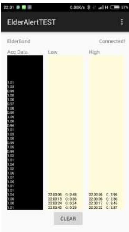
Figure 7 Acceleration data logged when fall occur
