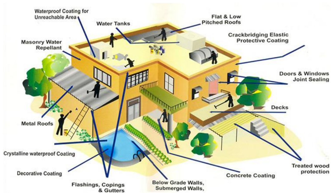
Figure 3. Complete waterproofing solution for a building
