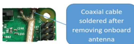
Figure 4. Coaxial cable soldered onboard
