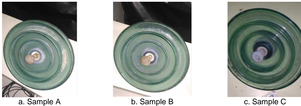
Figure 1. Glass insulator samples used in the experimental
