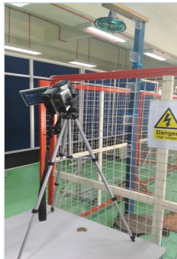
Figure 2. Experimental setup showing the thermal camera positioning
