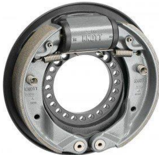
Figure 21: Brake System( Knott, n. d)
