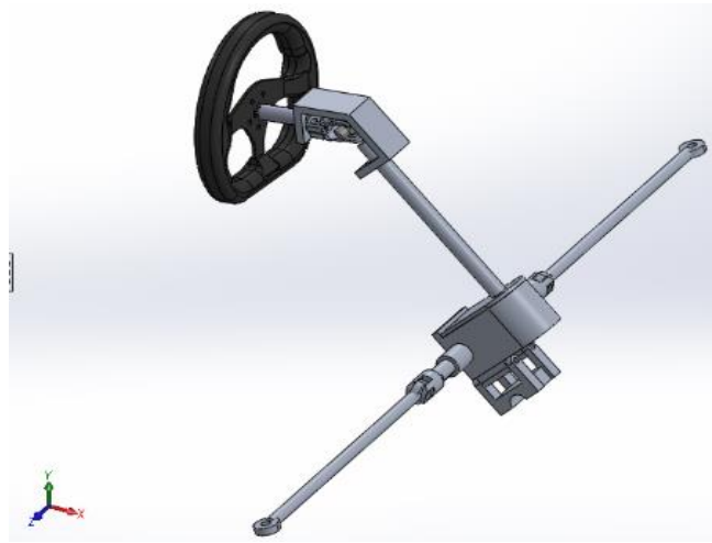
Figure 18: Ackerman Steering Model ( Ytingcom, n. d)
