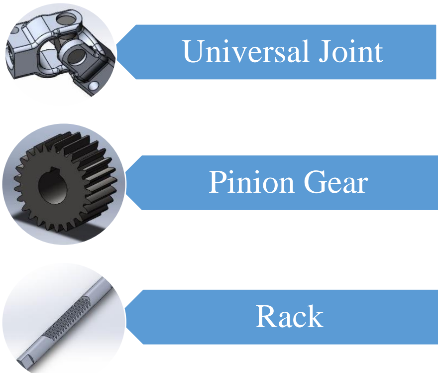
Figure 19: steering components ( Ytingcom, n. d)
