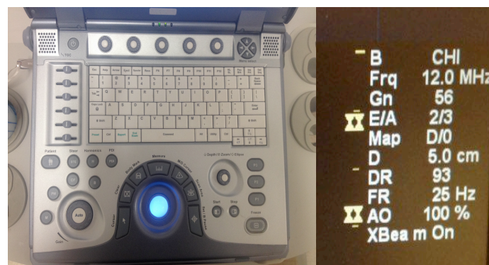
Figure 6: Example of ultrasound image parameters that can be manipulated to image optimisation. On the right side the display of this settings (frequency: 12 MHz; gain: 56; depth: 5.0 cm; dynamic range: 93). (Picture of LOGIQe equipment, General Electric Healthcare, GE Ultraschall, Deutschland GmbH & Co, Germany.)
