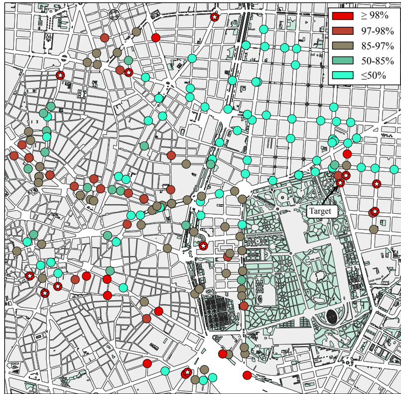
Figure 1: Automatic traffic recorders (ATRs) in the center of Madrid, colored by their data availability during 2014 (in % of valid 15-minute intervals over the year).
