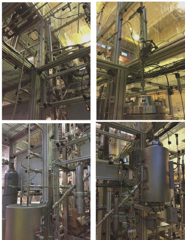
Fig. 5. Pictures of the installation used in this work. Bottom left: air reactor inside the electrical oven and loop seal. Left: riser with pressure sensors; top: cyclone; right: vessel and gate valve; bottom right: fuel reactor inside the oven and loop seal.
