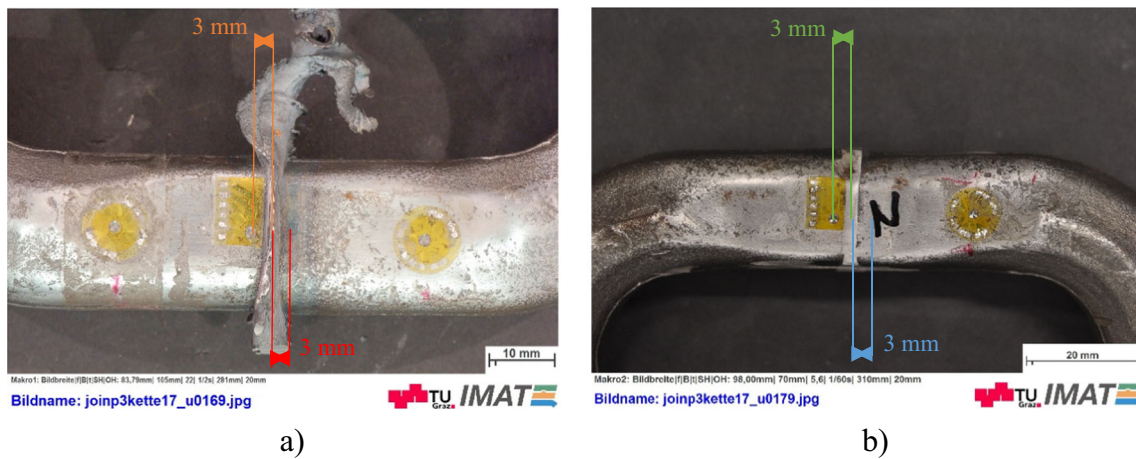
Fig. 9 Location of the measurements in the a A and b N conditions. TL 3 mm region
