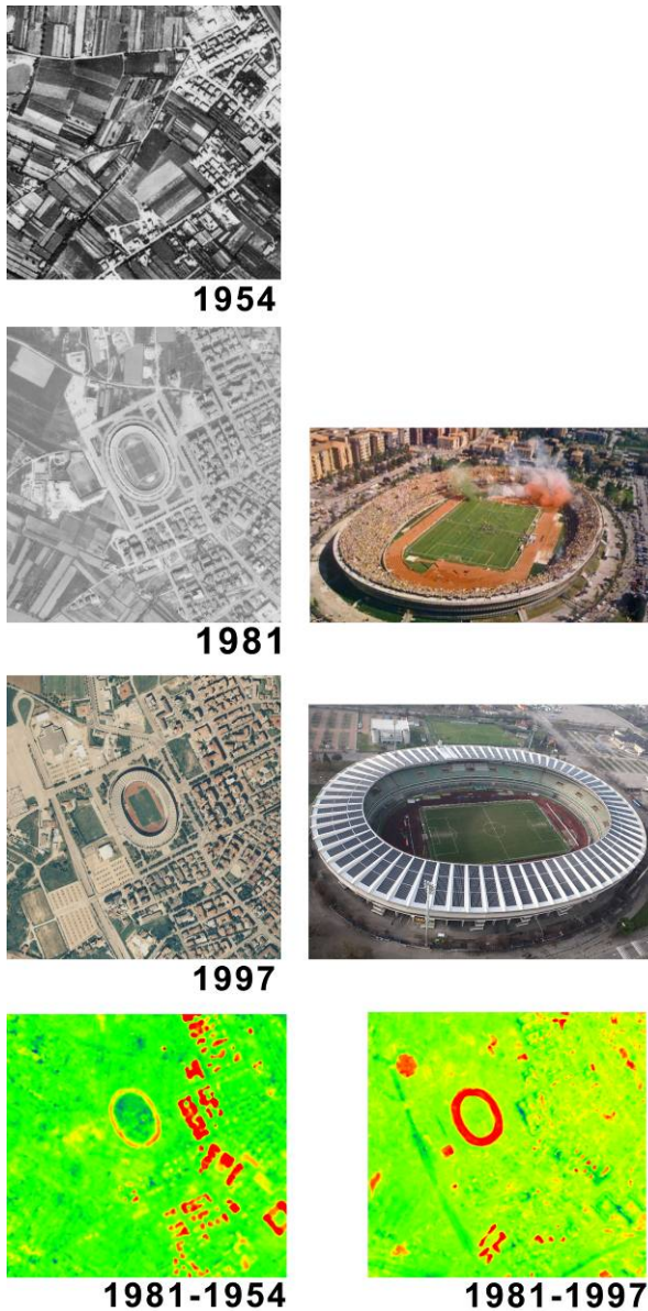
Figure 5: Example of city transformation documented by the comparison of 3d models of different period. On the left the extraction from orthofotos of the area of the Stadio Bentegoni in Verona. On the right two images of the stadio before and after changes. At the bottom the maps of differences
