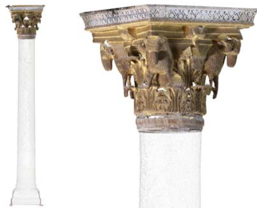
Figure 2: example of multiscale acquisition. The lower part of the column was acquired with 24 mm and the resulting point cloud has a less than 1 cm resolution. For the capital, acquired with 85 mm, the resolution is less 1 mm
