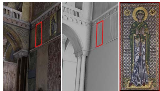
Figure 9: three products for the same area. From the left: textured mesh, NURBS model, Orthophoto
