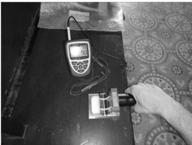
FIGURE 10 Calibration of probe sensor with test block for construction materials
