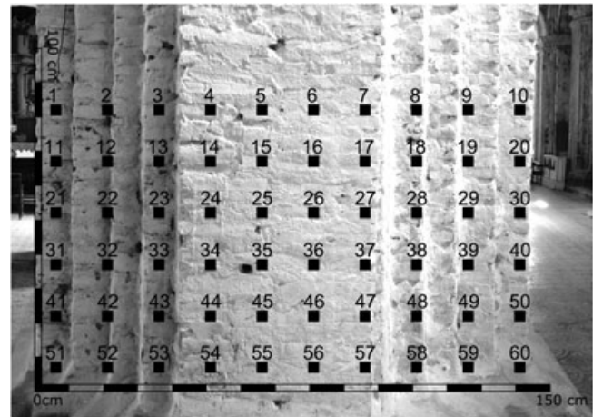
FIGURE 13 Displacement of the grid of points used for the direct sonic test on one cross-shaped pillar
