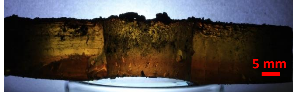
Figure 9. Cross section view of a fired VFP HTPB grain (Test No. 1, nozzle side). The grain profile shows a uniform contour, without anisotropies.
