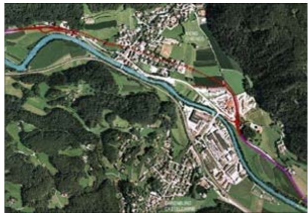
Figure 3. The longitudinal axis (red line) of the new tunnel to by-pass the village of Kiens/Chienes.
