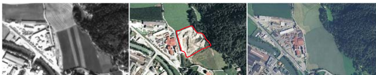
Figure 7. Patches from orthoimages (from left to right: 1986, 1995, 2006) depicting a portion of the territory of Kiens/Chienes in correspondence of polygon ID= 223 (in red on the central patch), where a covered former open pit has been found.
