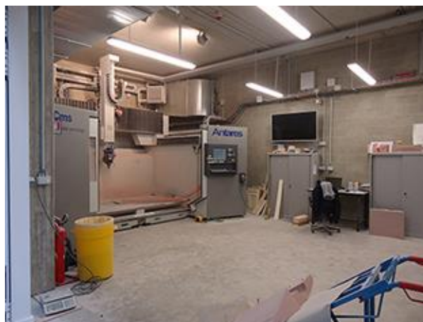
Fig. 12: Five axis CNC machine in Prototyping Laboratory.
