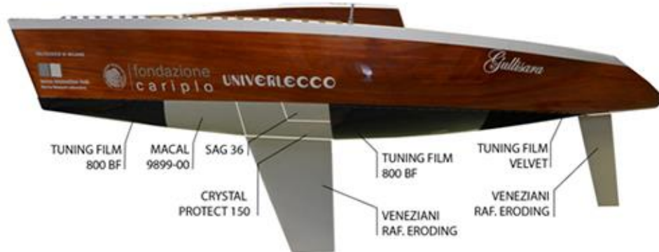
Fig. 19: Reference diagram to place the product samples on boat hull.
