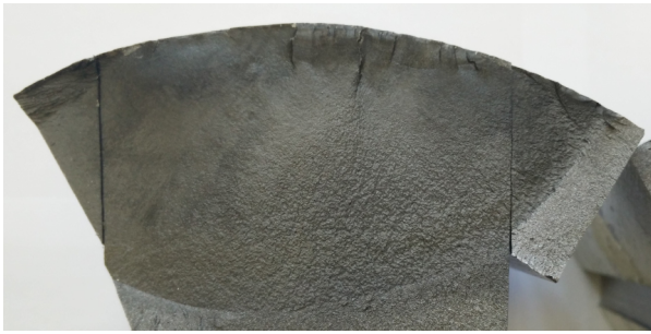
(a) Axle #1. Final failure at a micronotch. Maximum crack depth: 25mm
