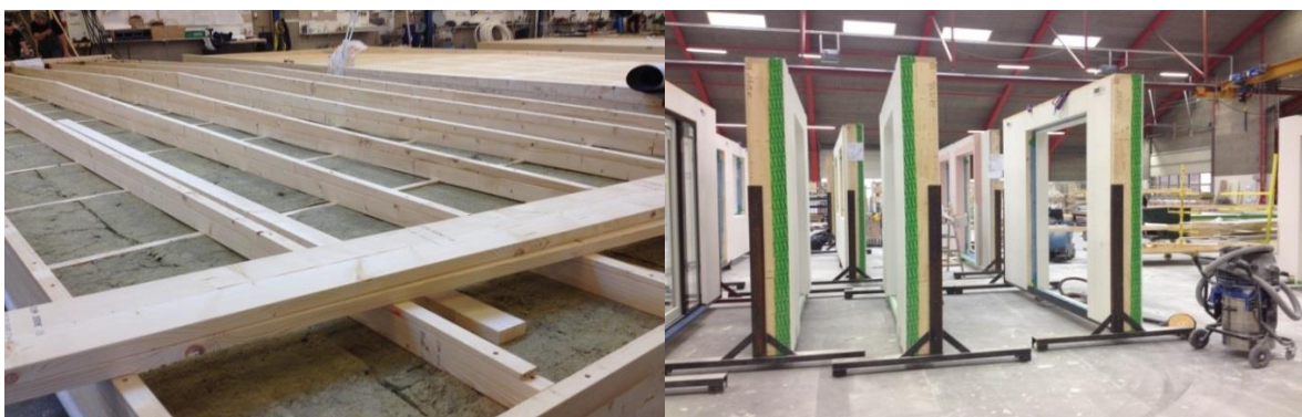
Figure 35. Wood is the primary construction material used, Scandi Byg, Denmark, workshop visited on 4 February 2014.
