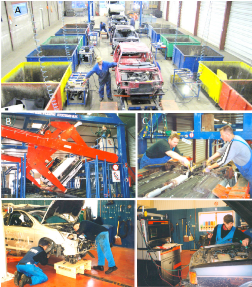
Figure 1. A-C: Examples of disassembly tasks from the present investigated serial-flow system where “end of life” cars are disassembled. D-E: Previously investigated traditional Swedish system.
