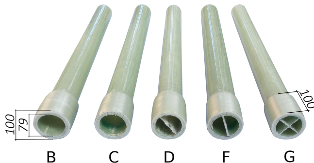
Figure 4: Selection of different manufactured cylindrical composite design concepts, where the inner area is visible.
