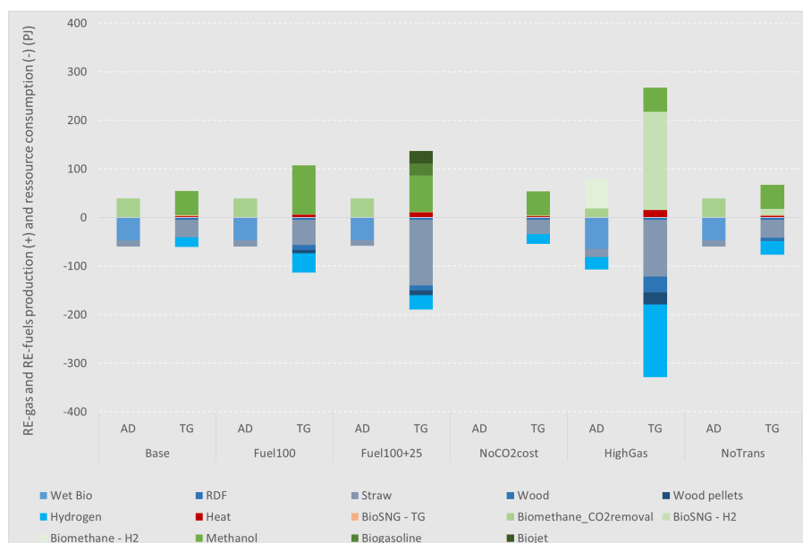
Figure 6: Danish RE-gas and RE-fuels production (+) and fuel consumption (-) by 2050 in the investigated future scenarios. AD: Anaerobic digestion; TG: Thermal Gasification
