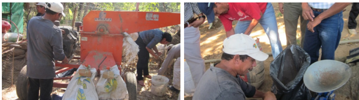
Grinding of ingredients to improve mixing. The weighing of the ingredients must be exact to avoid poisoning or digestive problems to animals (Photo: Jiménez-Trujillo, JA in 2013)
