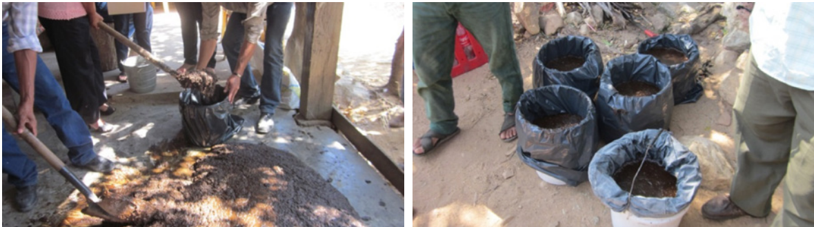
Figure 21. Introduction of the pasty mass and drying in the moulds
