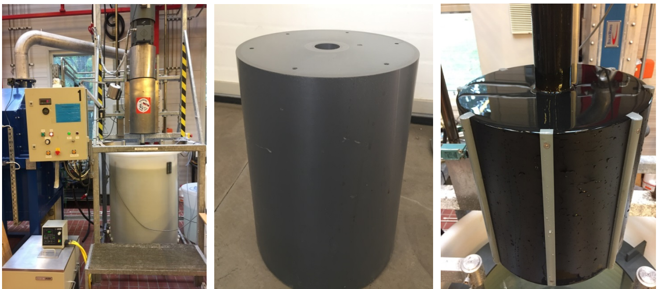
Figure 1. The full pilot-scale rotary setup for drag resistance measurements (left), cylindrical rotor (made of polyvinyl chloride) used in the rotary setup (shown without a coating applied) (middle) and the flexible rotor (made of polyoxymethylen) with six artificial welding seams (made of polyvinyl chloride, the grey parts in the photo) on the outer surface (right).
