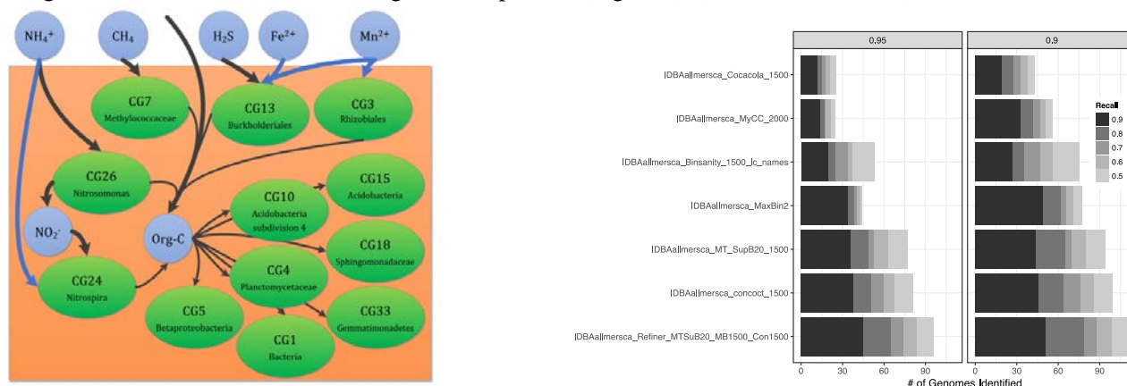
Figure 1. Left) Model of predicted metabolic and geochemical processes facilitating the degradation of groundwater contaminants in rapid gravity sand filters based on metagenomic analysis. Grey arrows denote certain metabolic capability while blue arrows denote putative metabolic capability. Right) Number of recovered genomes with seven different binning methods for a precision of 95% (left panel) and 90% (right panel). Recall denotes the completeness of the recovered genomes.
