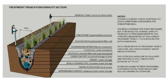
The figure illustrates one possible design of the Treatment Trench and its different components.
