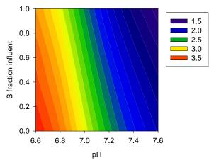
Figure 1: Influence of changing the pH vs. S (sulfate + sulfide) fraction in the influent on the reactor performance index (RPI) in M $\notin$ year. Point A = default conditions; point B = influent S is removed; point C = pH decrease to 6.8.
