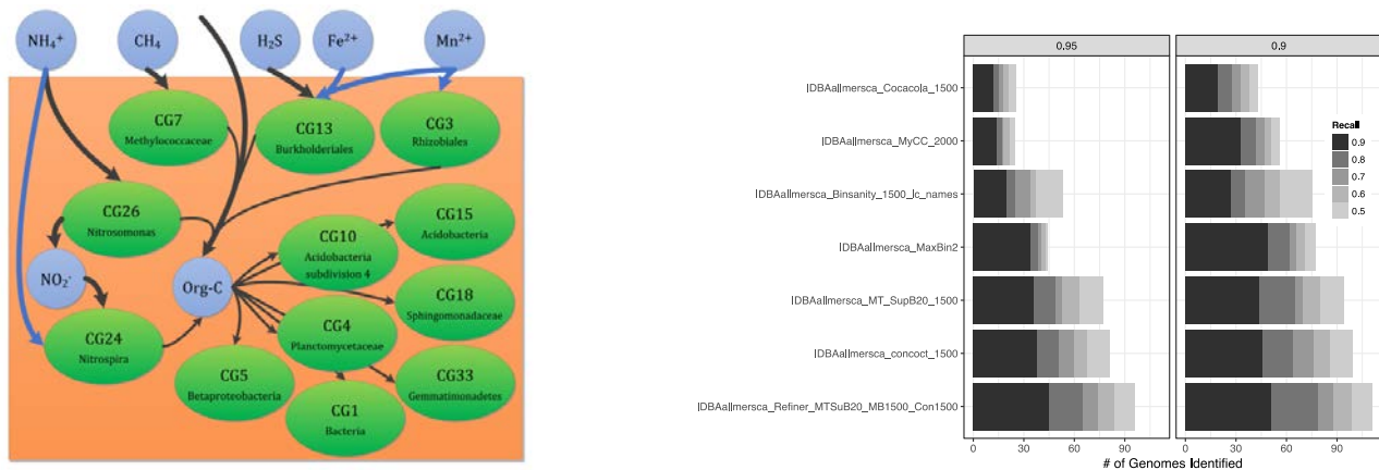
Figure 1. Left) Model of predicted metabolic and geochemical processes facilitating the degradation of groundwater contaminants in rapid gravity sand filters based on metagenomic analysis. Grey arrows denote certain metabolic capability while blue arrows denote putative metabolic capability. Right) Number of recovered genomes with seven different binning methods for a precision of 95% (left panel) and 90% (right panel). Recall denotes the completeness of the recovered genomes.
