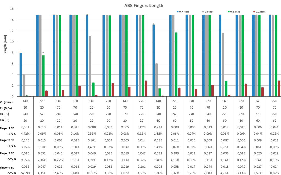
Figure 7. Average flow length of ABS on the four fingers for each DOE experimental run. Note 1: error bars on histograms indicate standard deviation (SD). Note 2: Coefficient of Variation COV% = average/SD × 100%.
