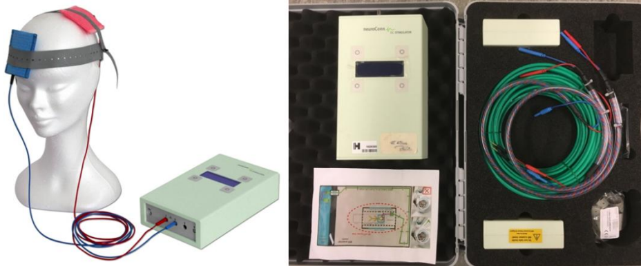
Figure 2.1: The employed MRI-conditional TCS device (DC-STIMULATOR PLUS, neuroConn, Ilmenau, Germany).
