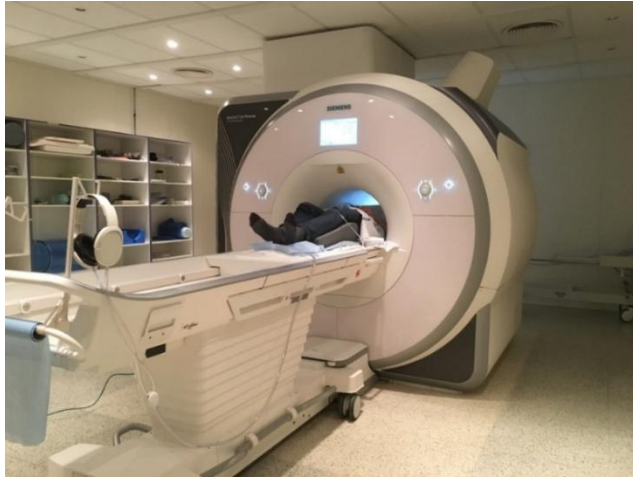
Figure 2.2: The employed 3T MRI scanner (PRISMA, Siemens Healthcare, Erlangen, Germany).
