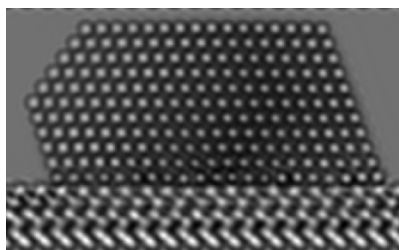
Figure 5.5: Simulated HRTEM image of a platinum nanoparticle on cubic \text{ZrO}_2 . The simulation parameters follows those used in section 4 with a defocus \Delta f = 8 nm.
